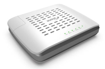
The 5225A is the next generation of 10Gbit ONTs designed for advanced triple-play deployments in home and business environments in a compact footprint. The SFP+ based uplink supports both symmetric 10/10 XGSPON and Active Ethernet technologies by simply swapping the optical transceiver.
