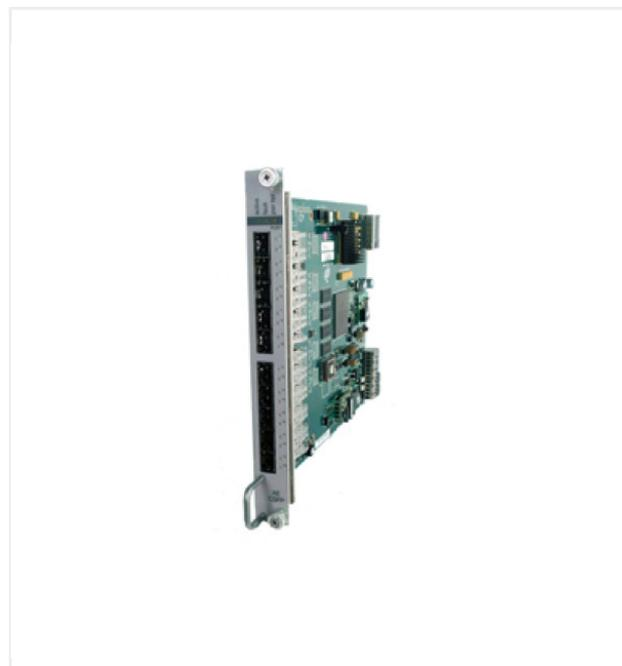
ports on the card can be used to support fiber services to 20 customers per card. The card also supports single channel SFP's for a total of 10 subscribers per card.
