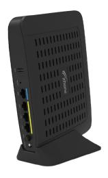
The 1764WC-A from Zhone with 2.5G WAN port is the ideal solution for extending wireless networks within the subscriber's premises. Exclusively designed for whole-home coverage, these Ethernet devices are equipped with dual-band 2x2 802.11ax wireless standard. Acting as an Access Point or a Mesh Client, the 1764WC-A is able to provide always-on connectivity and high-speed Internet with enhanced subscriber experience management.
