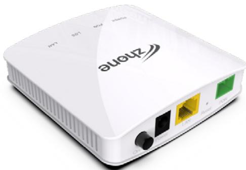
The 6201GN includes one SC/APC GPON interface, one 10/100/1000Base-T port. The ONT supports wire-speed L2 bridging and L3 gateway features, with carrier grade voice services.
