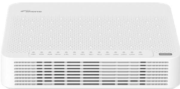
The Zhone H660GX includes one SC/APC GPON interface, four 10/100/1000Base-T ports, two FXS RJ11 voice ports, dual-band 2.4GHz and 5GHz wireless, and one USB compliant port. The ONT supports wire-speed L2 bridging and L3 gateway features, with carrier grade voice services using SIP VoIP protocols.
