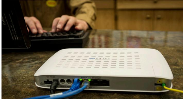
DZS zNID 2624P Optical Network Terminal (ONT) is unobtrusive and smaller than traditional telecommunications equipment.
